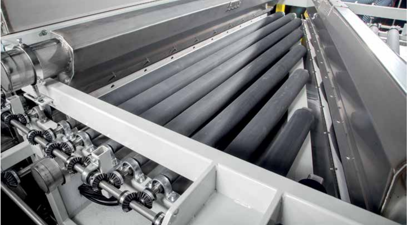
Washing area and drying blades in stainless steel. Air knives and water collecting slide in stainless steel.
