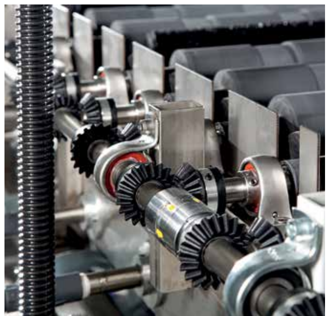
Transmission with conical gears in reinforced PA6, driven by a shaft in stainless steel, maintenance free.
